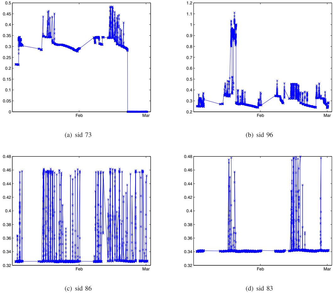
Figure 2. The soil moisture data collected by the first four sensors in the network during the months of January and February 2008. 'x' mark actual readings, and the y-axis show raw data collected by the sensor.
